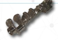
High performance automotive and aircraft engine crankshafts are nitrided for better fatigue resistance and wear properties on bearing journals.
