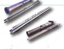
Life-enhancing and wear resistance improvement applications for plastic screw and barrels  Nitriding gears for applications ranging from heavy-duty machinery to small automotive accessories enables lower manufacturing costs. For one customer, this meant eliminating costly finishing operations needed after carburizing.
